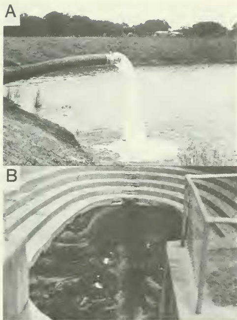
FIG. 2. Sampling nets placed on outlets of the G. Ligocky Well, Uvalde County (A) and Barton ("Concession") Springs, Travis County (B).
